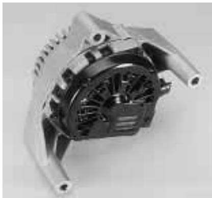
Figure 2. A version with long-arm mounts was introduced in 1996 on 3L V6 Taurus and Sable.
