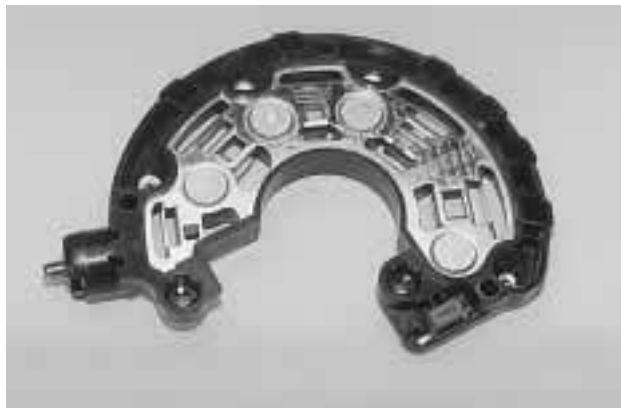
Figure 7. Sections of the copper heat sink are cut and bent over for better transfer of heat away from the rectifier.
