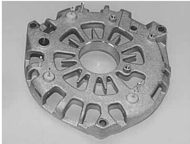
Figure 6. The three 50-amp negative diodes have white potting material. The 25-amp negative diode has black potting material.
